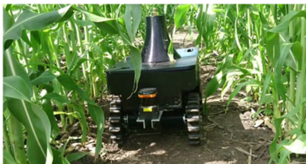
FIGURE 3 TerraSentia robot (0.31-m wide) in sorghum field. This crop has a nominal lane width varying between 0.76 and 0.91 m. A LiDAR Hokuyo UTM-30LX is positioned in the front part. LiDAR: light detection and ranging [Color figure can be viewed at wileyonlinelibrary.com ]
